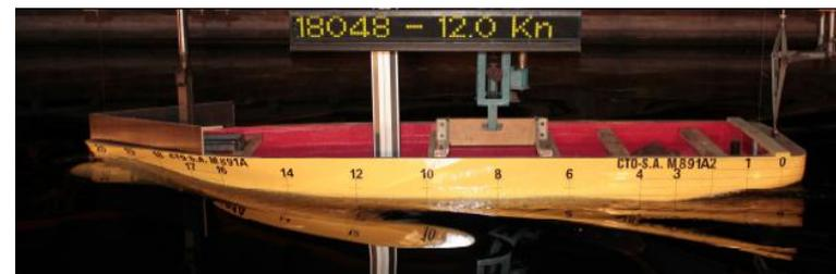
Still Water Resistance and Propulsion Tests
